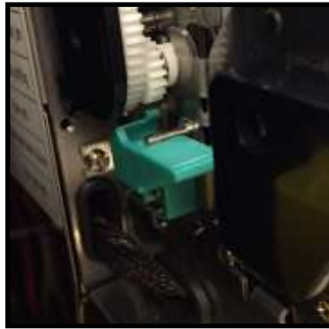
Figure 2: Green Release Latch
